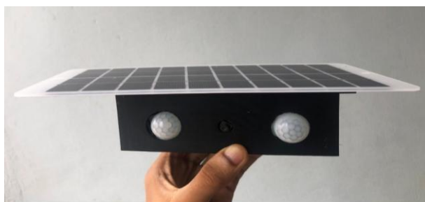
Figure 2. Front view of the developed anti-theft system prototype, showing the integrated camera, PIR sensor, and weatherproof enclosure designed for remote transformer security applications.
