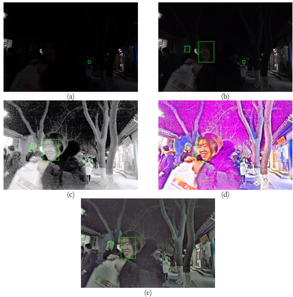
Figure 6. Detection with bounding box comparison of low-light face image enhancement methods (a) raw image; (b) CLAHE; (c) HE; (d) LIME; (e) LUMEN
