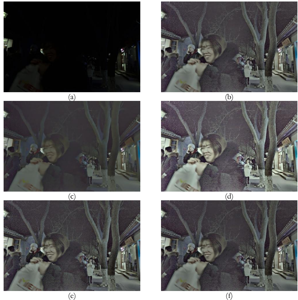
Figure 8. Visual comparison of low-light face image enhancement ablation (a) no retinex; (b) no AGC; (c) no CLAHE; (d) no fusion; (e) no denoising; (f) full configuration (LUMEN)
