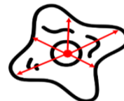
Figure 4. Amorphism Assessment Using Standard Deviation of Centroid-to-Vertex Distances
